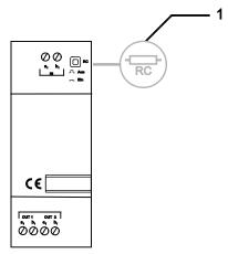
Fig. 2: Setting the terminal resistor on the device
